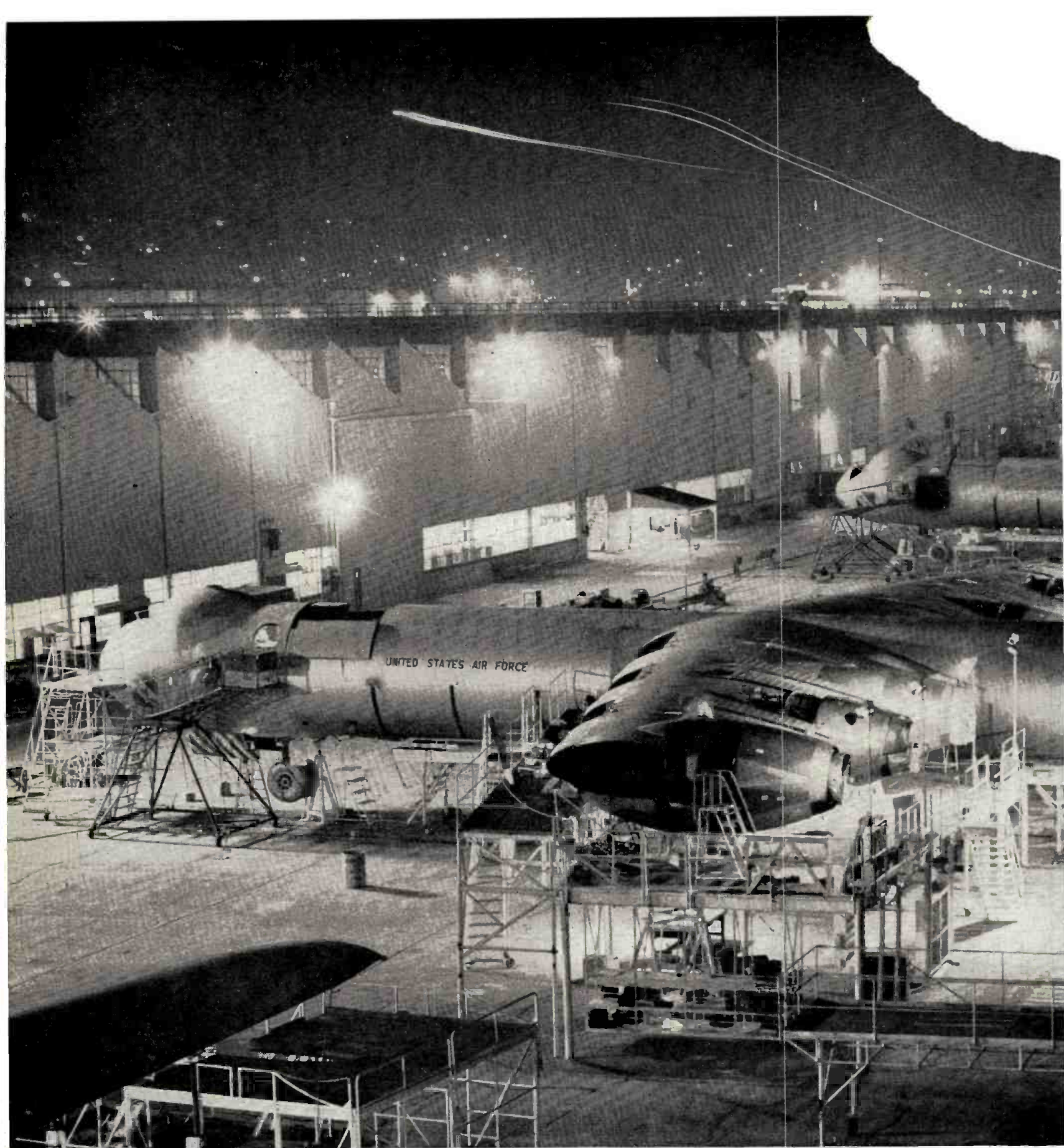
INSTALLING JET ENGINES IN B-36's, PICTURE TAKEN AT CONSOLIDATED VULTEE PLANT NO. 2 AT 1:30 A. M.
